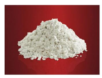
Superwool is manufactured from pure raw materials and processed to offer excellent performance in high-temperature applications. Superwool offers an alternative to traditional solutions due to its high refractoriness and excellent non-wetting characteristics with molten aluminum.
